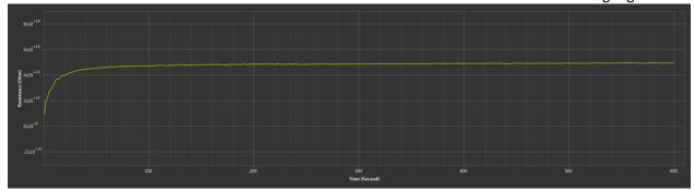
Test ID = Test Point 2 Test Voltage/Current = 500V IRt1 = 49.41GΩ IRt2 = - PI/DAR = -
