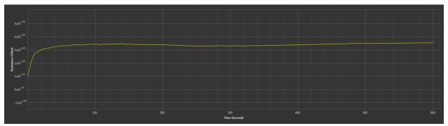
Test ID = Test Point 1 Test Voltage/Current = 500V IRt1 = 35.51GΩ IRt2 = - PI/DAR = -
