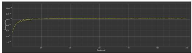
Test ID = Test Point 6 Test Voltage/Current = 500V IRt1 = 16.30GΩ IRt2 = - PI/DAR = -
