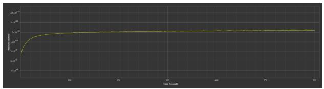
Test ID = Test Point 3 Test Voltage/Current = 500V IRt1 =  $15.95G\Omega$  IRt2 = - PI/DAR = -
