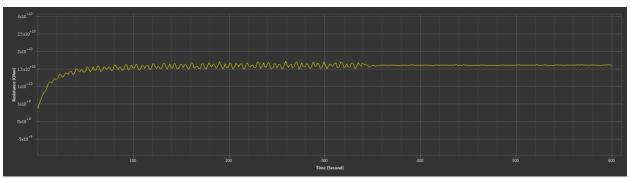
Test ID = Test Point 4 Test Voltage/Current = 500V IRt1 = 16.13GΩ IRt2 = - PI/DAR = -
